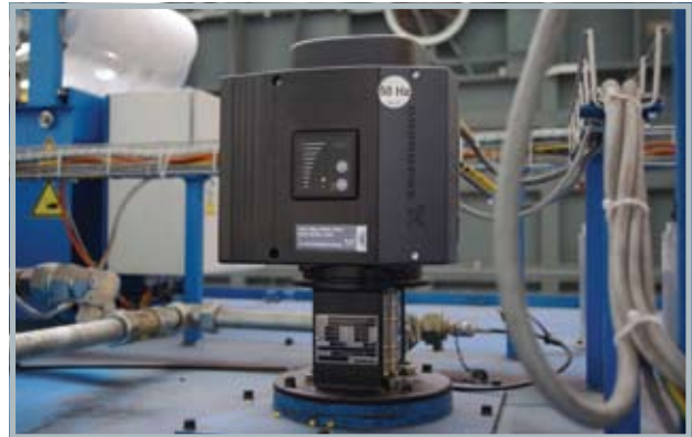
MTRE pumps are vertical multistage centrifugal pumps designed for pumping of cooling lubricants for machine tools, condensate transfer and similar applications. MTRE pumps are fitted with an E-motor, i.e. a motor with built-in frequency control.
