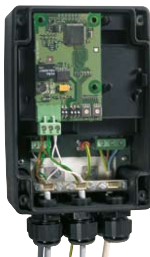
CIU 200 Modbus interfaces enables the pumps to be monitored and controlled centrally.
