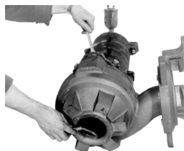
Fig. 14 Measuring the impeller clearance
