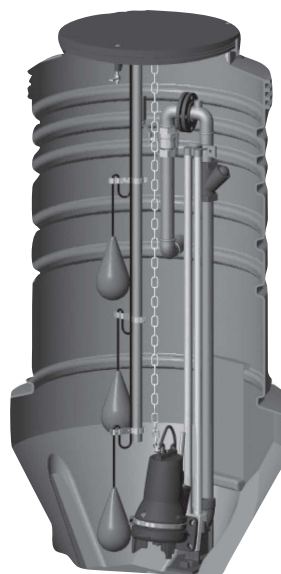
Pit with pump on auto coupling with goose neck outlet
