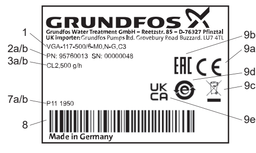
Nameplate of a VGA-117 dosing regulator
