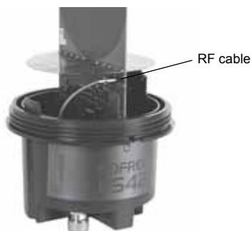
Fig. 5 Connecting the RF cable
