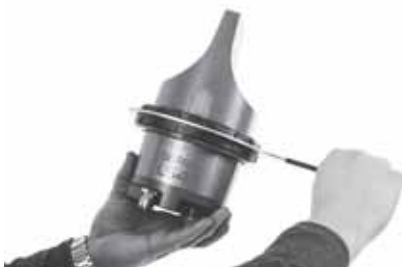
Fig. 2 Removing the top cover
